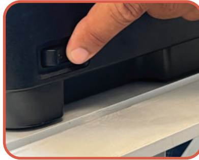
14. PRESS THE SWITCH ON THE BOTTOM RIGHT SIDE OF THE PRINTER TO TURN IT ON.
