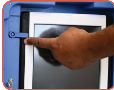
8. UNLATCH THE TABLET USING THE BLUE LEVER.
