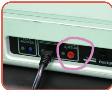
15. PRESS THE RED BUTTON ON THE BACK OF THE TW TO TURN IT ON.
