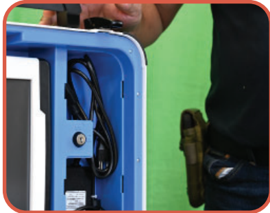
7. REMOVE THE POWER CORD FROM THE STORAGE COMPARTMENT. CLOSE THE COMPARTMENT AND CASE.
