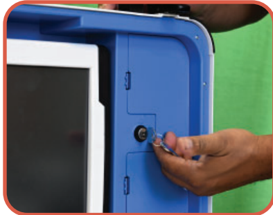
7. UNLOCK THE TABLET USING THE YELLOW/RS KEY.
