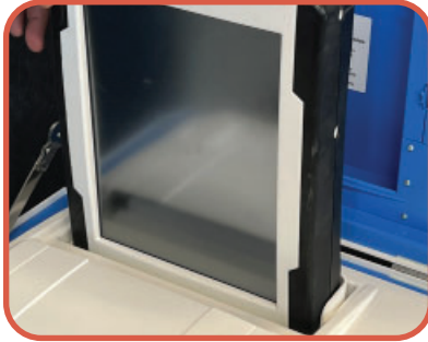
13. SEAT THE TABLET IN THE CRADLE AND TILT IT BACK.
