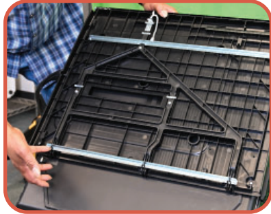
7. RELEASE THE LID BY UNHOOKING THE THREE STRAPS.
