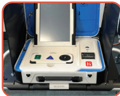
17. ATTACH PRIVACY SCREENS TO THE SIDES OF THE ADA STAND.
